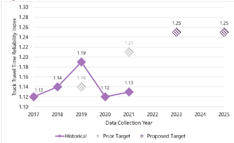
Figure 2: Interstate truck travel time reliability index – historical condition, prior targets, and proposed targets
